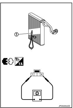
If NG, replace intake sensor. Refer to <u>VTL-12. "Removal and Installa-</u> tion". INFOID:000000004215321
