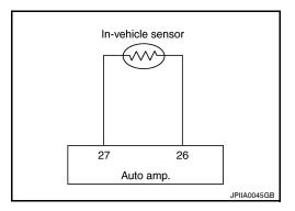
In-vehicle Sensor Circuit
