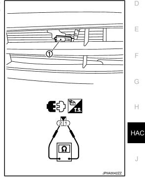
If NG, replace ambient sensor. Refer to <u>VTL-11, "Removal and</u> <u>Installation"</u>.
