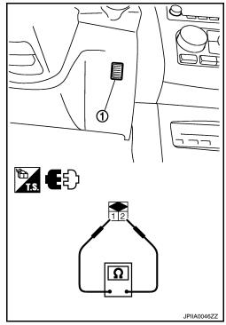
If NG, replace in-vehicle sensor. Refer to <u>VTL-9</u>, "Removal and Installation"
